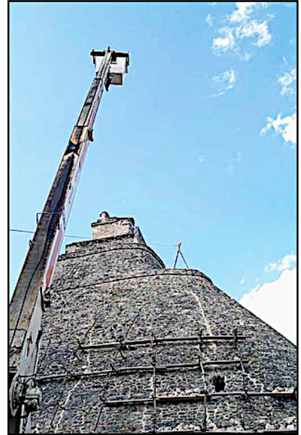
Figure 24. Hydraulic lift with survey camera team photographing the south side of the pyramid. Pic: Roberto Centeno L., 1999.
