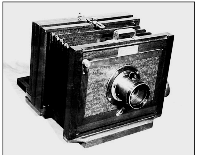
Figure 11. Scovill view camera similar to the camera used by the Le Plongeons. Single lens could be replaced by dual lenses for 3D stereo photos. Pic: L. G. Desmond, 1985.
