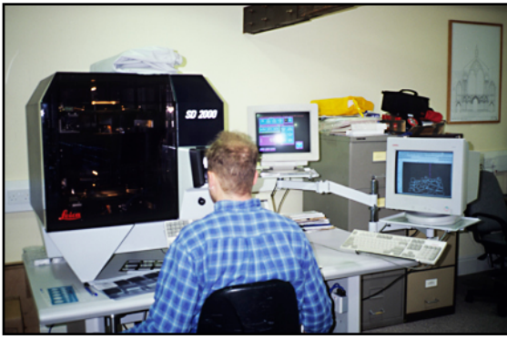
Leica SD2000 stereoplottter. Pic: L. G. Desmond, 2000.
