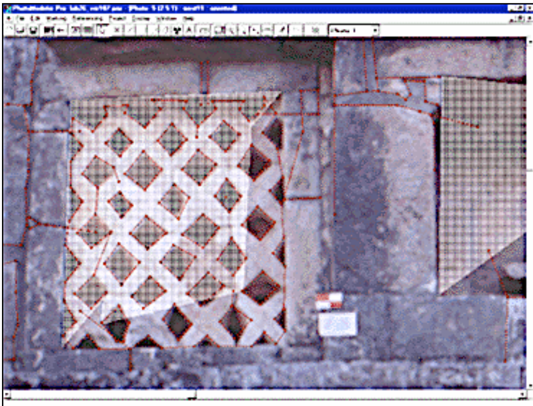
Fig. 6. All the points and lines generated in PhotoModeler.
