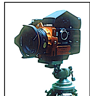
Bronica camera remanufactured as a calibrated photogrammetric camera by American Measuring Instruments of San Antonio, Texas. Pic: L. G. Desmond, 1989.
