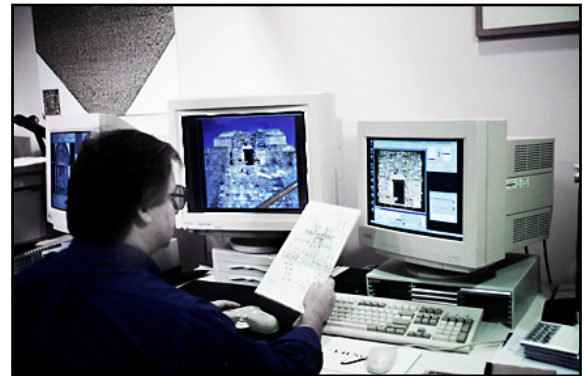
Michael Clowes working in a 3-D environment to generate an orthophotograph of the Chenes Temple with the Leica Helava all digital photogrammetric work station. Pic: L. G. Desmond, 2000.
