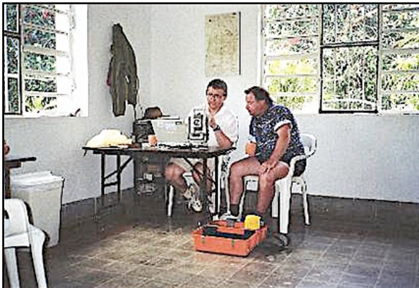
Paul Bryan and Mick Clowes downloading survey data from the total station surveying instrument to a laptop computer in the archaeology laboratory at Uxmal. Pic: L. G. Desmond. 1999.
