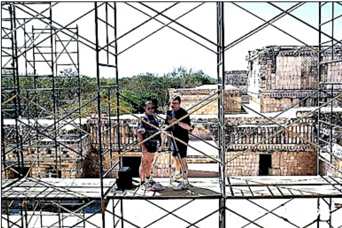
Photos of the west facade were taken in stereo 3-D by moving the camera in the horizontal plane along the scaffold. Photos are being taken from the first platform 7 meters above the ground with a Rolleiflex 6006 camera by Mick Clowes and Paul Bryan. Pic: Roberto Centeno Lara. 1999.
