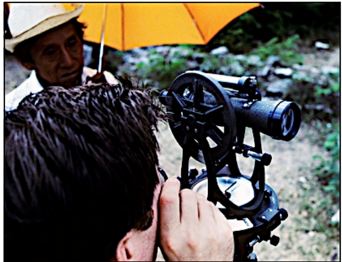
Survey transit accurate to 30 sec. of arc was used to determine 3-D coordinates of targets on La Iglesia and the Adivino Pyramid for the 1989 photogrammetry project. Pic: L. G. Desmond. 1989.
