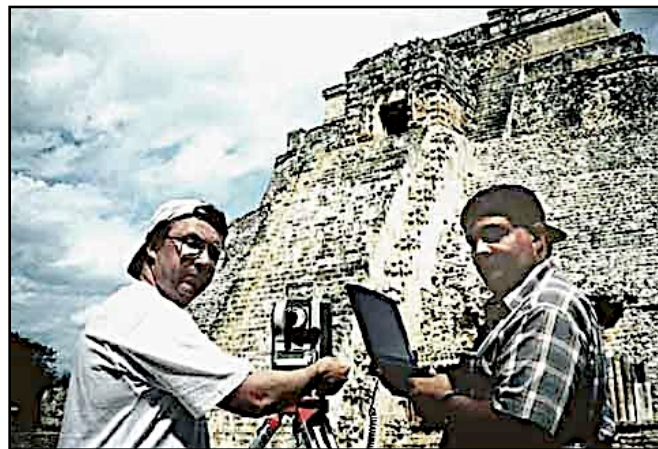
Paul Bryan and Francisco Mendoza surveying the west facade of the pyramid. Laptop computer for storage of data from the total station. Pic: L. G. Desmond. 1999.
