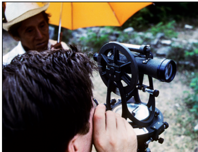
Transit accurate to 30 sec. of arc was used to determine 3-D coordinates of targets on La Iglesia, and the Adivino Pyramid for the 1989 photogrammetry project. Pic: Lawrence G. Desmond, 1989.
