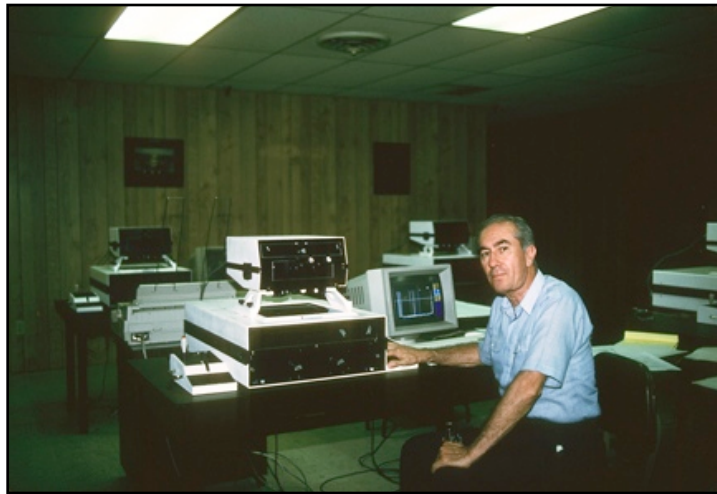
Photogrammetrist John Garcia with American Measuring Instruments 35/70 Stereoplotter at AMI offices in San Antonio, Texas. Pic Lawrence G. Desmond, 1990.
