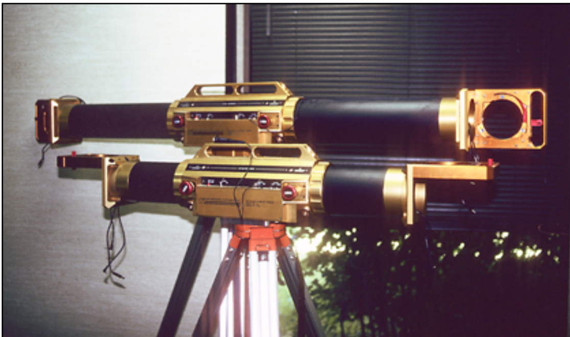
American Measuring Instruments twin bar photogrammetric units for photographing architecture without the use of survey targets. Pic: Lawrence G. Desmond, 1989.
