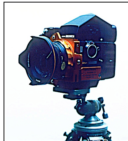
Bronica 70mm camera remanufactured as a calibrated photogrammetric camera by American Measuring Instruments of San Antonio, Texas. Pic: Lawrence G. Desmond, 1989.
