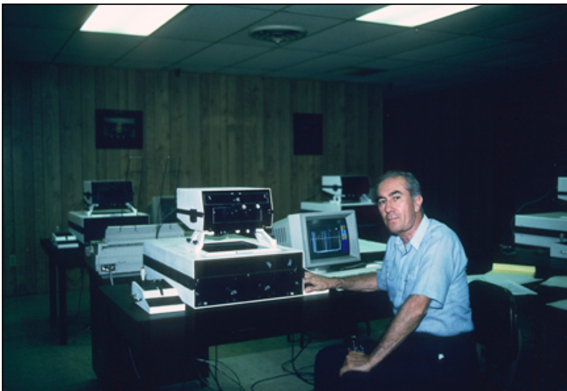
Photogrammetrist John Garcia with American Measuring Instruments 35/70 stereoplotter at AMI offices in San Antonio, Texas. Pic: Desmond, 1990.
