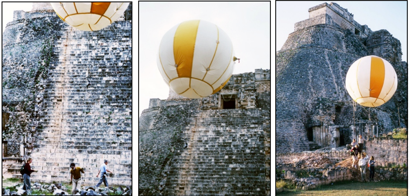
Hydrogen balloon with camera hanging below photographing the west facade of the Adivino Pyramid. Right photo shows balloon being walked to north and east sides for additional photos. Pic: Desmond, 1990.
